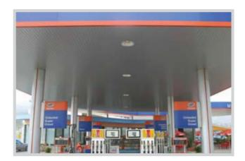
STAMPA linear ceiling available in 100 and 150mm. Produced of aluminium, plain or perforated, is installed onto carrier and provides a wide range of colours.
