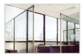
Open space - low height partitions are composed of vertical aluminium frames. Produced with various filling materials, offer unlimited choices and solutions in space formation needs.
